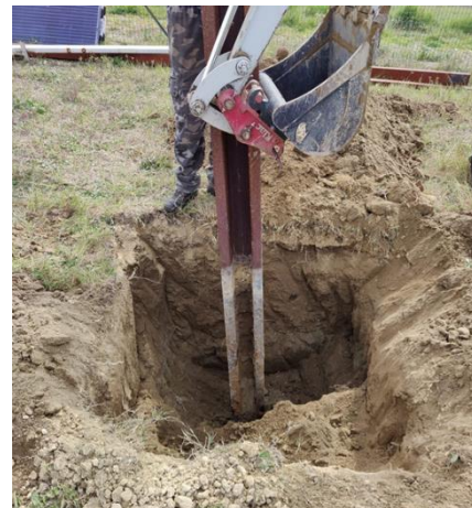
Figure 7 - A phase of the survey performed in Tuscania on the tracker piles
